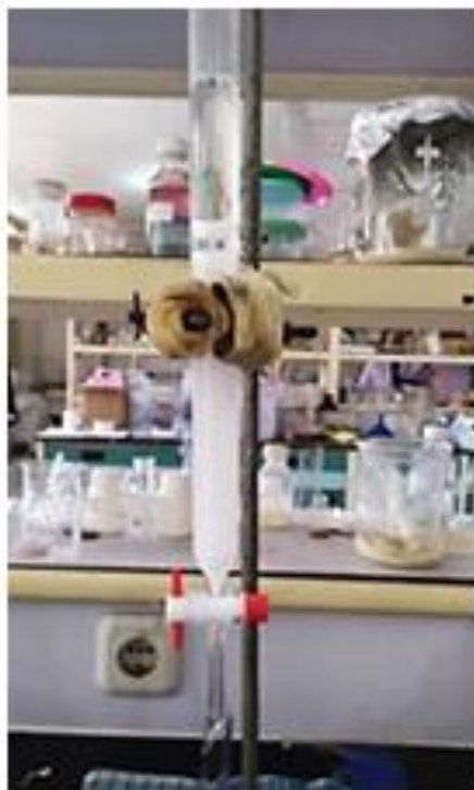
Figure S3: Fractionation using the stationary phase sephadex LH-20 (Source: Photograph courtesy of Syaiful Bahri. Copyright 2021)
