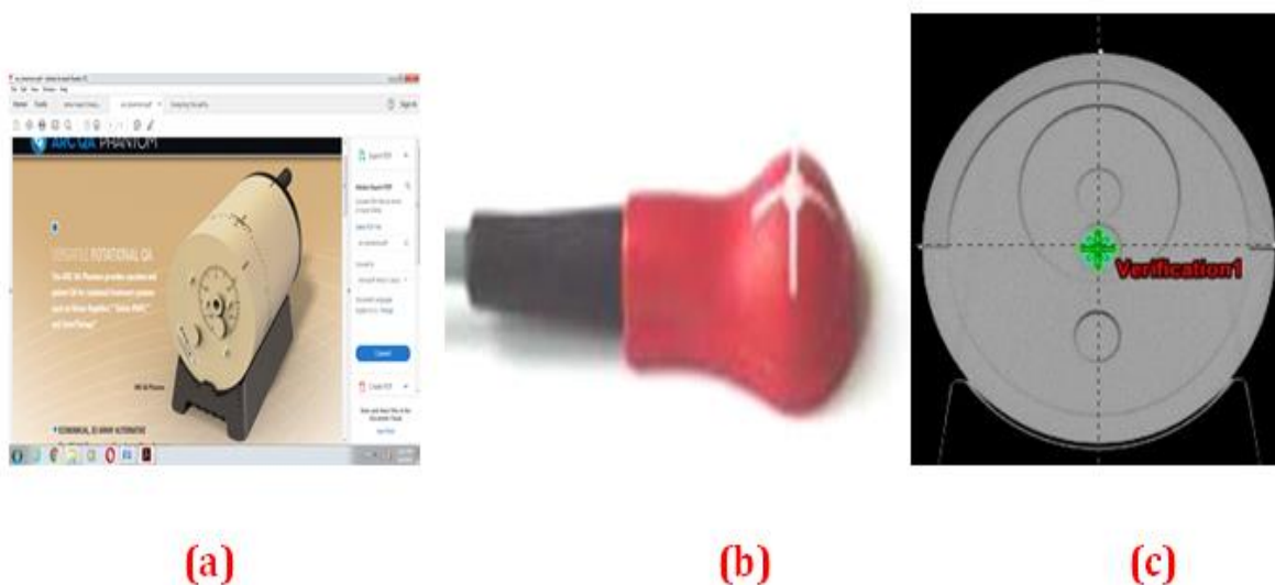
Figure 3: (a) Arc Phantom, (b) EDP-15 p-type diode, and (c) axial view
