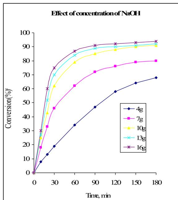
**Fig 3.** Effect of concentration NaOH.
